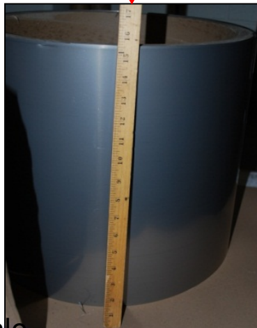
UTRC 6 mil foil subscale brazed heat exchanger 15" wide, 4 mil AFA foil for Solar Turbines (foil by Elgiloy) recuperator (Metalwerks 2000lb heat, Haynes, Somers, Elgiloy)
